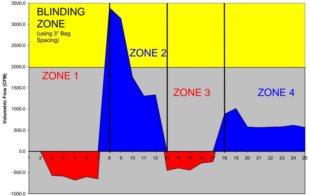
Figure 6. Blinding Zone with Generic Baghouse 3" bag spacing.
