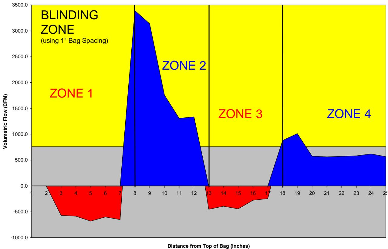
**Figure 4. Blinding Zone with Generic Baghouse 1" bag spacing.**
