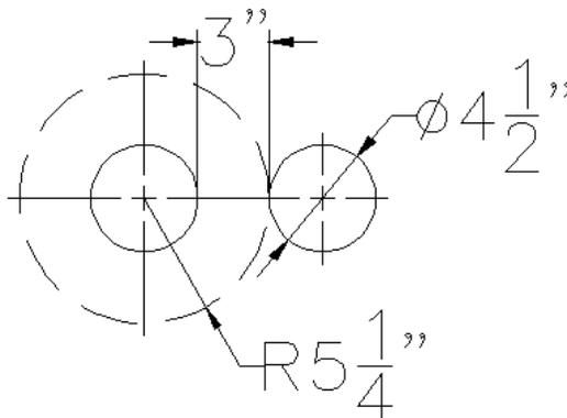
**Figure 5. Scientific Dust Collectors 3" bag spacing.**
